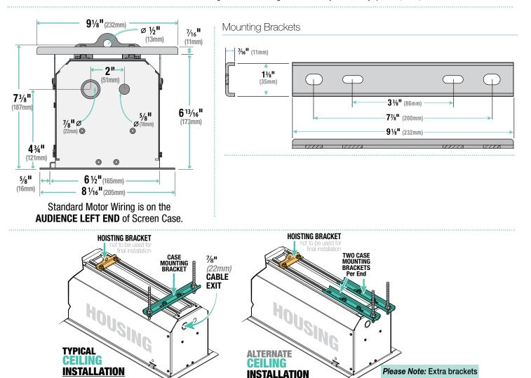
With typical installation, brackets may be angled to meet installation requirements.
