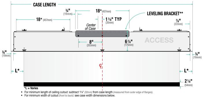
• \*\*Leveling bracket is used to level the case and should NOT be used to support the weight of the unit.
