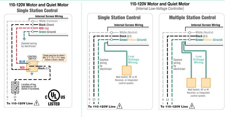
Wiring External LVC-IV to Motor
